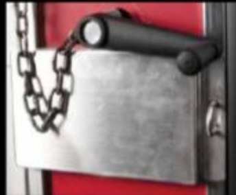
Heavy gauge chain secures the crank handle.
